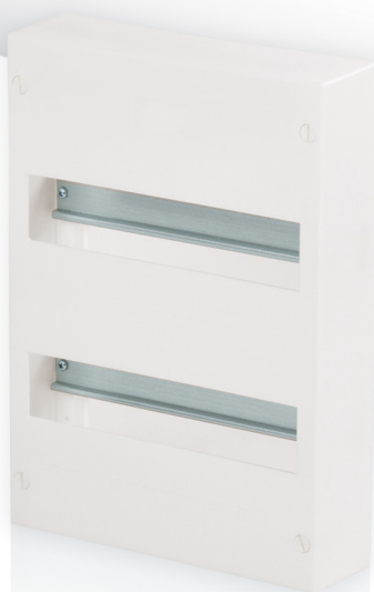
name N 24 A type IP 40 □ In 63A dimensions 353 x 250 x 70 number of modules 24 + 4 PE, N terminal 2 x 13
